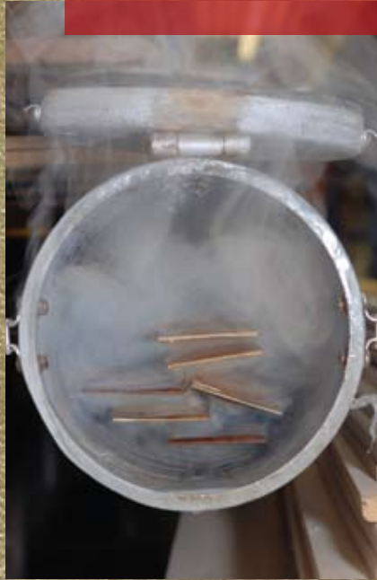
Various Hoop timbers in the steamer.
