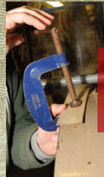
Starting a flesh hoop on the “wheel”, another custom-made piece of equipment. For all the hoops, the timber is taken straight from the steamer and turned on the wheel, then clamped and held in position with G clamps. Speed is of the essence when turning timber on the wheel, as the wood is more malleable or supple whilst it is still hot and fresh from the steamer. The cooler the timber gets, the harder it is to manipulate into shape.
