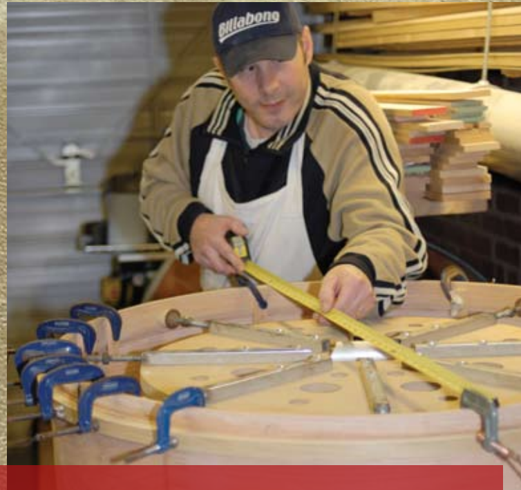
The centre hoop is fitted to one half of the shell. The diameters of the shell and centre hoop are checked. This drum's diameter is 3ft ¼ inch. This is the preferred size of shell, as any increase in diameter larger than this makes it more difficult to find sufficient quality goatskins to match to the drum.
