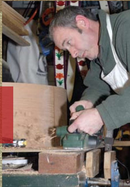
“Scarving” the oak centre hoop timber. This process ensures that the two ends of the timber merge neatly after being bent into shape.
