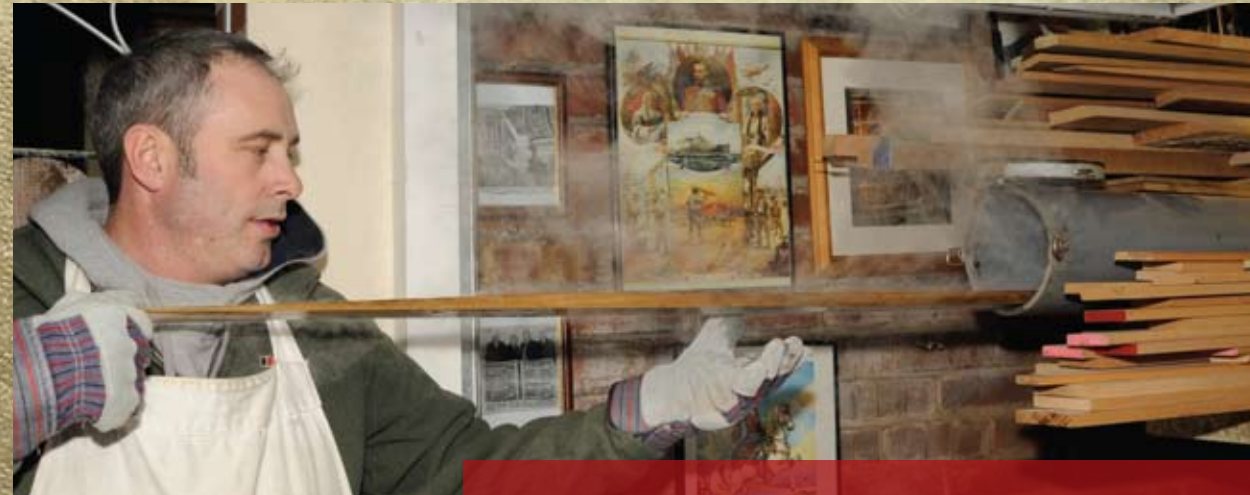
Removing hoop timber from steamer. (Note how the end is tapered or “scarved.”) The timber is extremely hot and needs to be handled with gloves to protect the hands.
